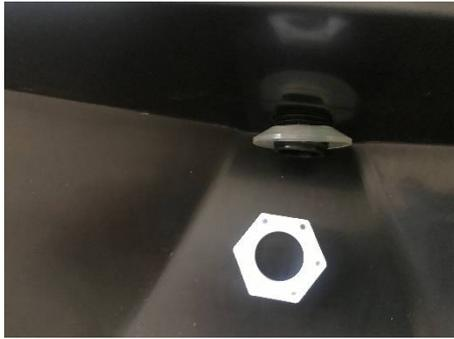
c. Put in the seal and tighten nut
